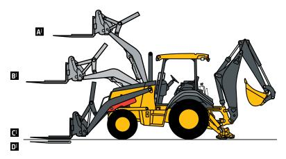
Lift capacities are over-end values in kg (lb.) according to SAE J31. Figures listed are 87% of the maximum lift force available. Base vehicle includes counterweight.
