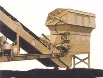
Tine type shredder is designed for use in top soil and other related materials.
