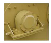
All TRIO Washers utilize lower outboard grease lubricated, anti-friction, self-aligning spherical roller bearing assembly with replaceable rubber "donut" seals and stainless steel wear sleeves. The mounting of the bearing outside the tub protects the bearing from water and dirt, and provides easy inspection and fast maintenance access.
