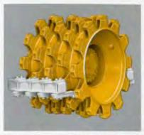
Wheels with tamping foot design and modified chevron pattern give traction, penetration and compaction needed for high production. Modified chevron patterns are reversed on front and rear drums for one-pass double coverage: rear feet hit areas missed by front feet. Feet are anchored to drum with a continuous weld for extra strength. Each foot has replaceable weld-on tips.
