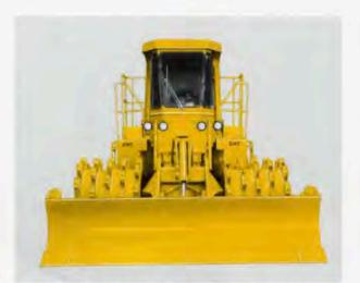
Fill-spreading blade is multiple box-section steel. Reversible cutting edges and self-sharpening end bits add service life.
