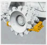
Two cleaner bars per wheel keep drums free of carry-over dirt...regardless of rolling direction. Cleaner tips peel — rather than shear — material. Adjustable and reversible for long life, tips can be replaced individually or as a unit.
